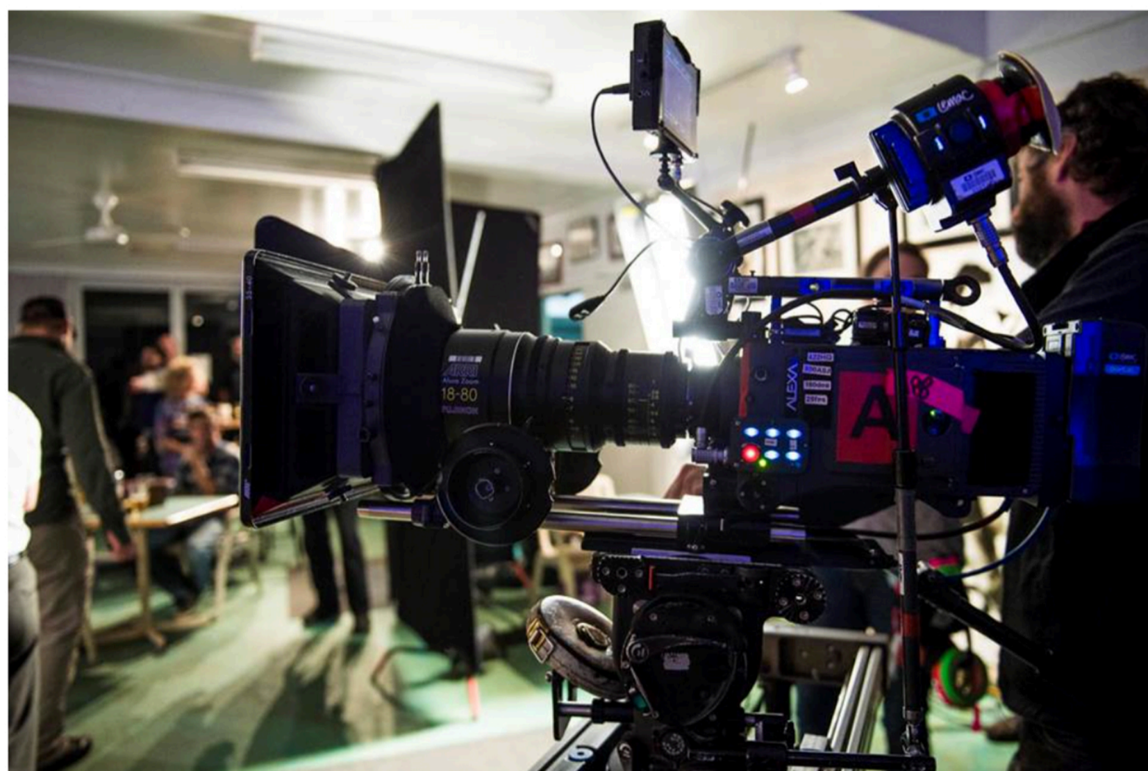
‘A’ Cam - Arri Alexa with Alura 18-80mm zoom with FF-4 follow focus, MB-18 mattebox, TV Logic reference monitor atop O’Connor 2575 head on the Grip’s slider.
